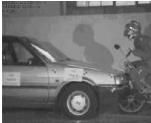
Fig. 5.3-8. Motorcycle frame starts to deform (time t = 0,054 s from the moment of first contact).
