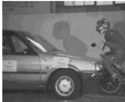
Fig. 5.3-9. Maximum deformation of the frame (time t = 0,068 s from the moment of first contact).
