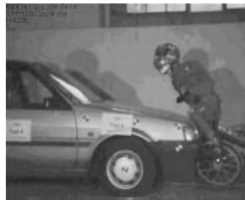
Fig. 5.3-10. Contact between the dummy and the handlebars (time t = 0,106 s from the moment of first contact).
